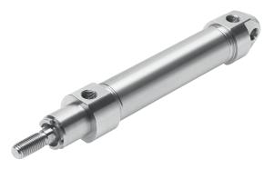
Preventing the development of infection sources on the Festo stainless steel round cylinder CRDSNU: a threadless design can be used for the bearing cap to reduce the risk of contamination in typical applications. In addition, the self-adjusting end position cushioning system (PPS) is designed without adjusting screws, which are susceptible to contamination.
